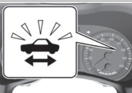
A photograph of the instrument cluster. A callout box shows a car icon with a double-headed arrow below it, indicating the vehicle is ready to start.                                                                                      |
