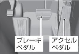
A photograph showing the driver's footwell area. Two lines point to the brake pedal and the accelerator pedal. Labels below the image read 'ブレーキペダル' (Brake pedal) and 'アクセルペダル' (Accelerator pedal).                                      |
