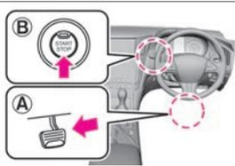
A photograph of the driver's seat and dashboard. A red circle labeled 'B' highlights the power button on the dashboard. A red circle labeled 'A' highlights the brake pedal. Red dashed circles highlight the driver's feet on the pedals. |
