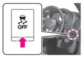
A photograph showing the VDC OFF switch on the center console and a circular callout highlighting the steering wheel with a pink arrow pointing to the center. |
